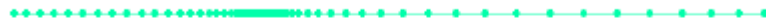
Figure 4.2: Grid points on the connectors are clustered towards the location of the backward step.
