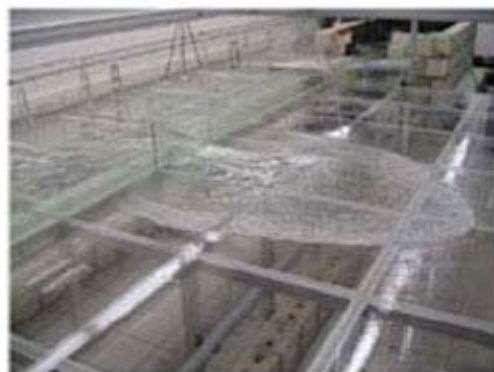
Figure 1. Sample flood wave in physical model
