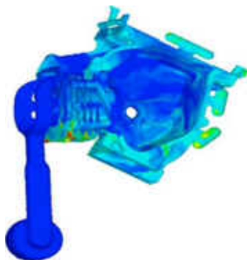
Figure 2: Air volume fraction (max 5%) including air drift and air escape at surface
